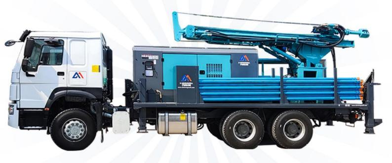
The MWT-250 vehicle-mounted water well drilling rig uses a new SINO HOWO truck chassis and is equipped with a 22 bar two-stage compression high-pressure air compressor. Its lifting force can reach 17 tons, and it can drill water wells with a maximum depth of 250 meters.
